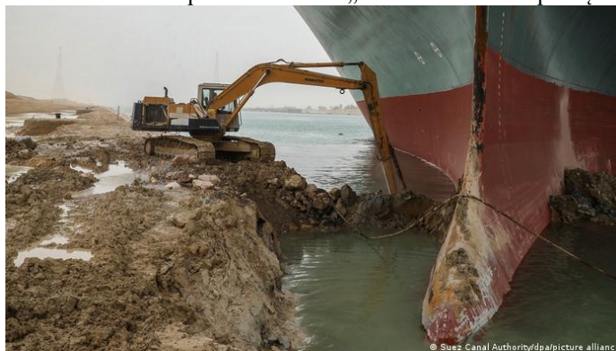
2 pav. Ekskavatorius atkasa konteinerinio laivo įstrigusį priekį ( https://www.dw.com/en/suez-canal-blockage-4-of-the-biggest-trade-chokepoints/a-57020755 )
